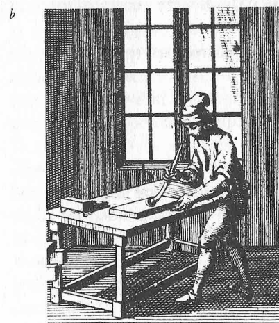
FIG. 68 (a, b). Bindery work in eighteenth-century France. (a) Sewing and ploughing; (b) finishing with a roll. ( Encyclopédie , planches viii, Paris 1771, 'Relieur', pls. 1, 5.)
