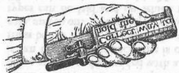
FIG. 3. A modern composing-stick. The size of the type is, of course, greatly exaggerated in order to show the faces.
